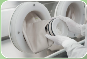
1. Pull the Glove/Sleeve outside the isolator.
