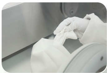
9. Working with one hand in the adjacent glove, carefully pull the old glove.
