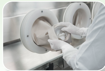
8. Put the glove/sleeve inside the isolator.
