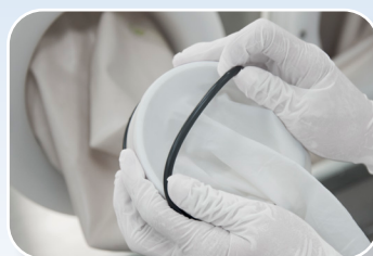
6. Install the ring up to the middle groove.
