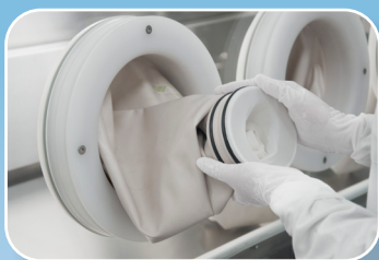
1. Pull the Glove/Sleeve outside the isolator.
