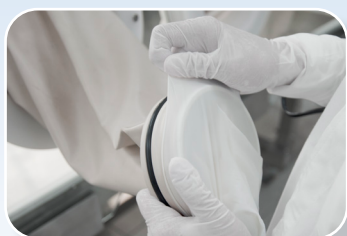
5. Take the new glove and ensure the thumb is at the top. Stretch the ring of the new glove over the port and over the old glove onto the middle groove.
