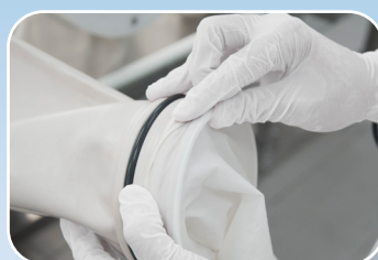
4. Carefully roll the gloves from the middle groove to the outer groove.
