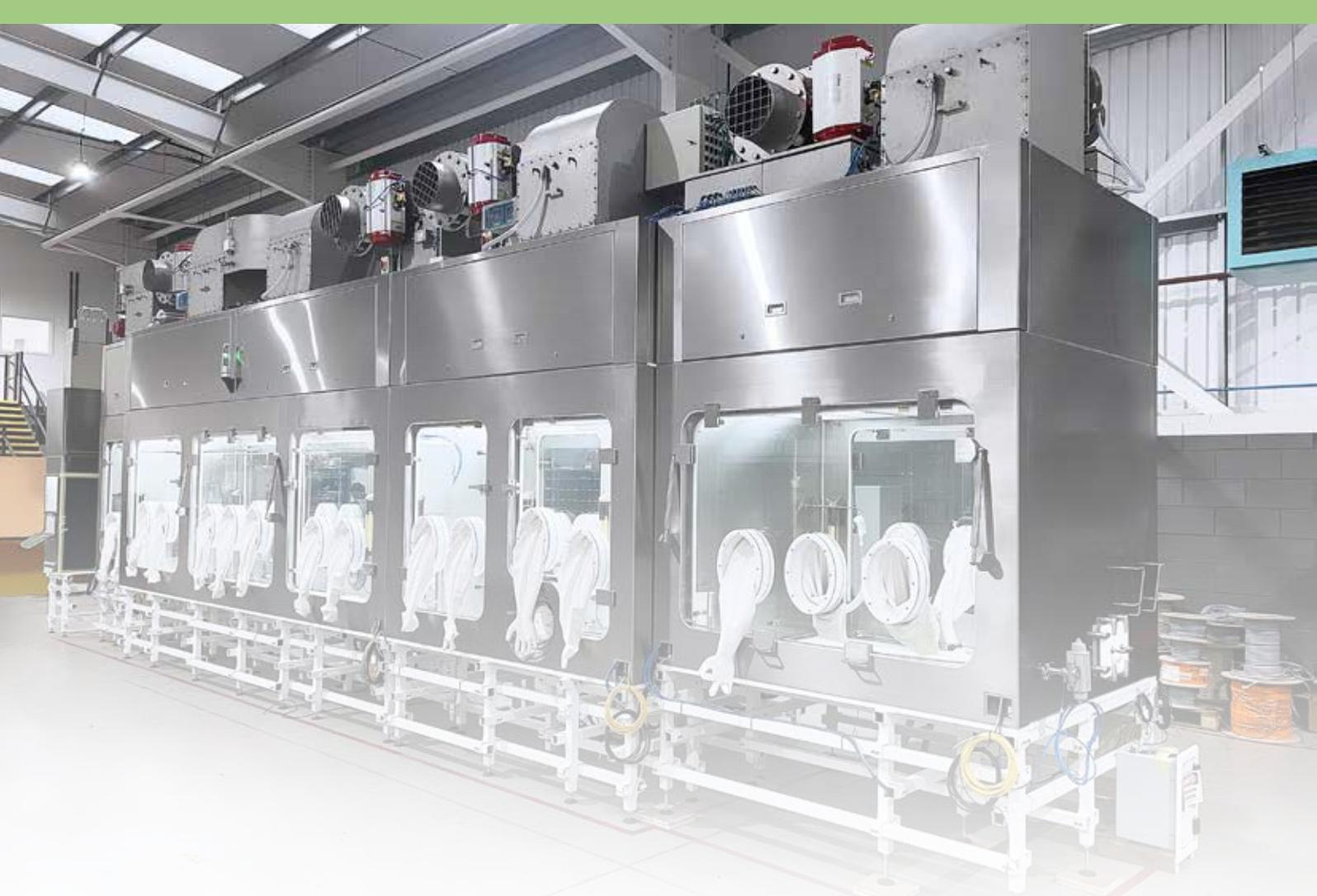
Filling lines enclosed in an isolation technology are now widely utilized for the aseptic manufacture of sterile pharmaceuticals in various container formats. Esco Pharma's filling line isolator provides an ISO Class 5 / Grade A environment, ensuring the sterility of the work zone for the most demanding sterile/aseptic operations.
