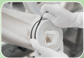
3. Remove the outer ring.
