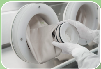
1. Pull the Glove/Sleeve outside the isolator.
