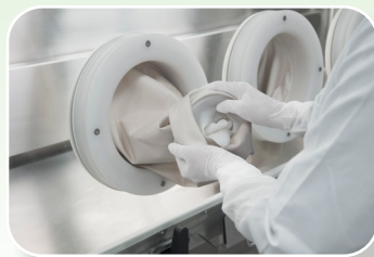
8. Put the glove/sleeve inside the isolator.
