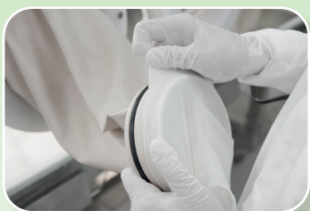
5. Take the new glove and ensure the thumb is at the top. Stretch the ring of the new glove over the port and over the old glove onto the middle groove.
