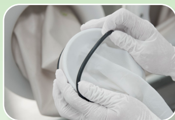
5. Take the new glove and ensure the thumb is at the top. Stretch the ring of the new glove over the port and over the old glove onto the middle groove.
