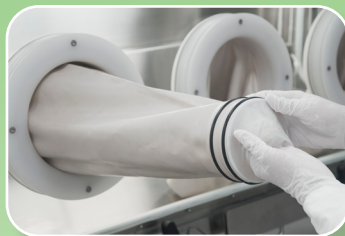
2. Fold the fingers of the glove inside the cuff ring.
