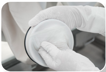
7. Carefully loosen the old glove from the outer groove.
