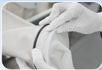
4. Carefully roll the gloves from the middle groove to the outer groove.
