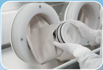
1. Pull the Glove/Sleeve outside the isolator.
