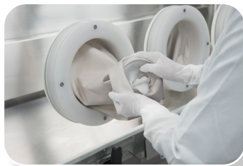
8. Put the glove/sleeve inside the isolator.
