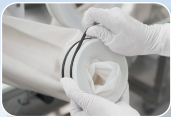
3. Remove the outer ring.
